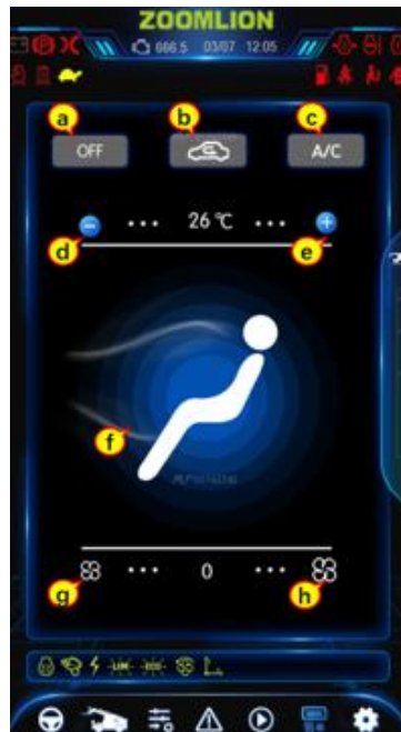
Figure 2-17 Air condition interface
