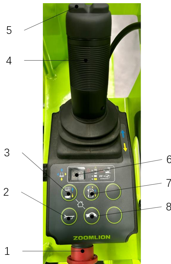
Figure 2-5 Platform control panel
