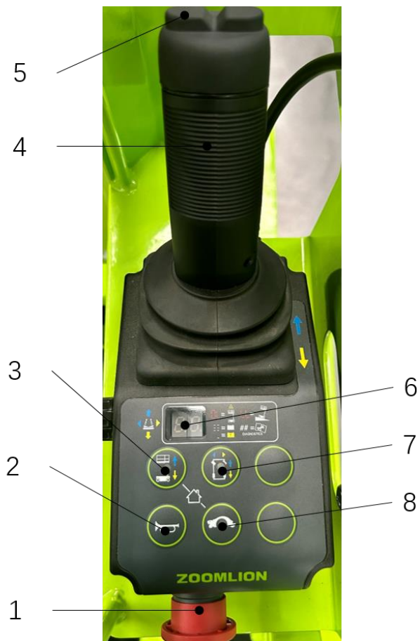
Figure 4-3 ZMP04/ZMP05/ZMP06 Platform control panel
