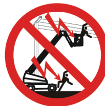
Figure 03 Minimum Safe Approach Distance
