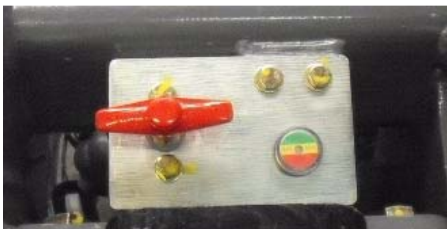
Battery charging indicator
