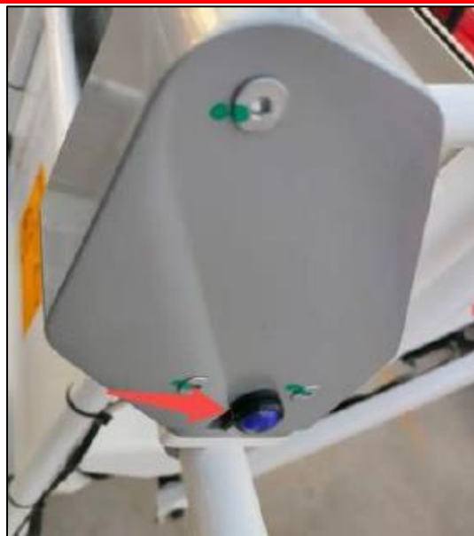
Figure-The Strobe Flashes Blue
