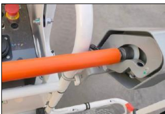
Figure-SPD Activated State
